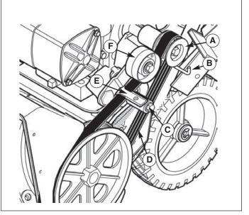
Figure 14. Drive Belt Installation
